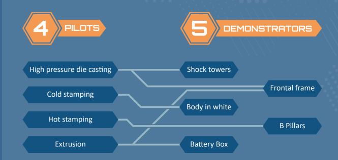
SALEMA is developing brand new aluminium alloys with low critical raw materials, but high recycled aluminium content. Each will be tested at four pilots and used in five demonstrator car parts manufactured for electric vehicles.
