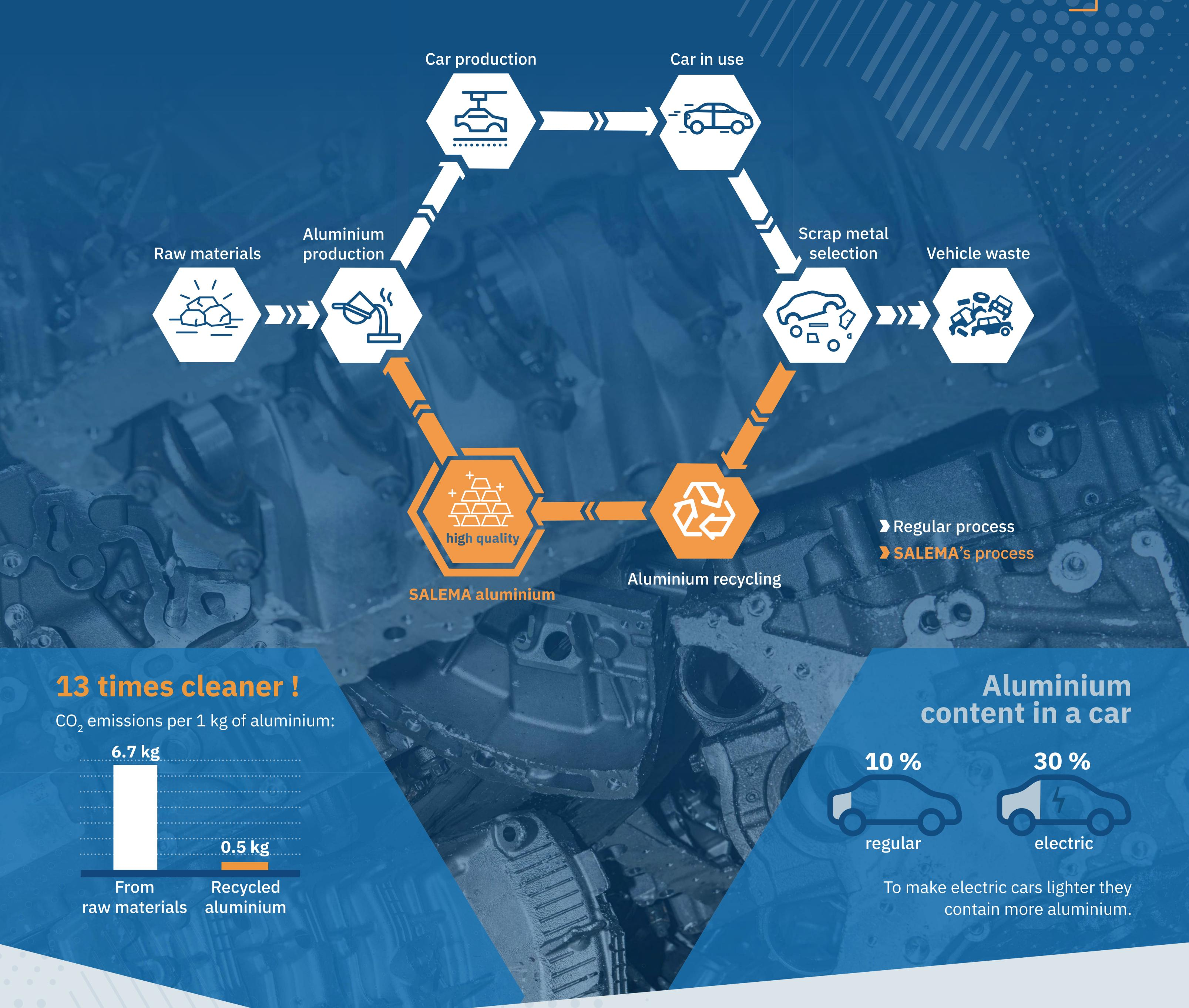
SALEMA developed brand new aluminium alloys with either low critical raw materials or high recycled aluminium content. Each was tested in four pilots and used in five demonstrator car parts manufactured for electric vehicles.
