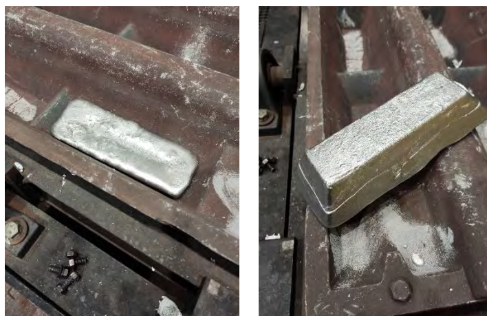
Figure 5. Images of the ingot mould used and one of the ingots cast
