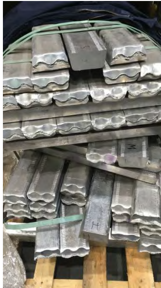
Figure 2. Image of the ingots supplied by Raffmetal for WP1 trials related to HPDC alloys
