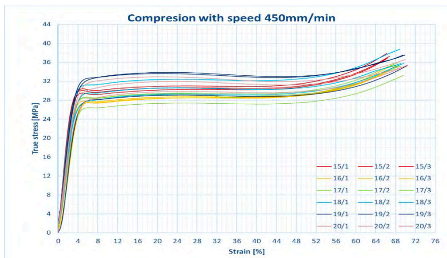
Figure 42. True stress-strain curves from compression test with crosshead speed 450mm/min.
