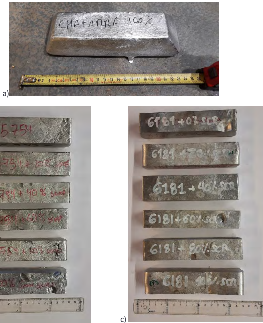
Figure 45: Ingots cast using the sheet metal compositions with increasing scrap contents: a) as-cast ingot; b) and c) samples machined from a plate of 5754 and 6181 with scrap contents 0%, 20%, 40%, 60%, 70% and 100%.
