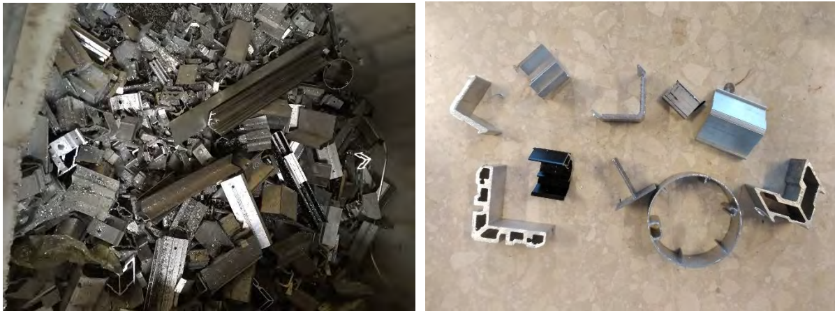
Figure 33: General overview of the 6063 extruded profile acquired from a local aluminium recycling company (left) and image of the 10 parts selected for a Spark Plasma chemical analysis (right)
