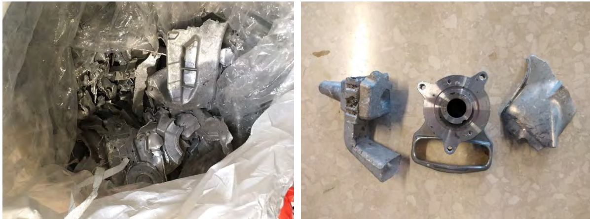
Figure 3: General image of the foundry scrap provided by Raffmetal (left) and image of 3 parts selected to conduct a chemical analysis by spectrometry (right)
