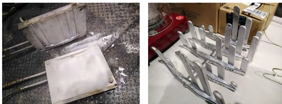
Figure 6. Pictures of the mould used for the fluidity test of the casting alloys and some of the samples obtained
