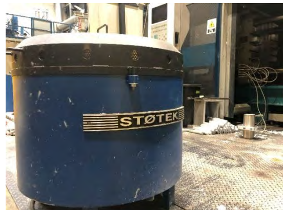
Figure 1. Stotek furnace, with a crucible with a capacity of 50 kg of aluminium, used to melt the material of WP1 tests
