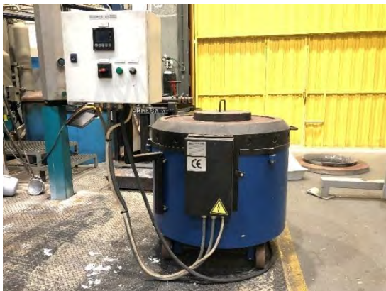
Figure 1. Stotek furnace, with a crucible with a capacity of 50 kg of aluminium, used to melt the material of WP1 tests
