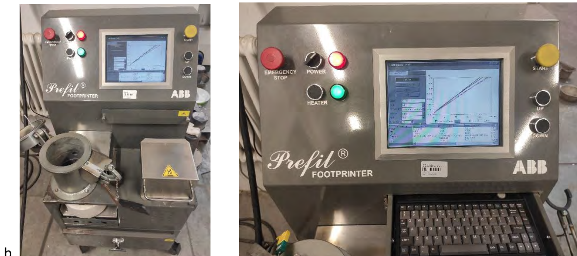
Figure 7. Sampling scheme for analyzing inclusions (a.) and PREFIL apparatus (b.)
