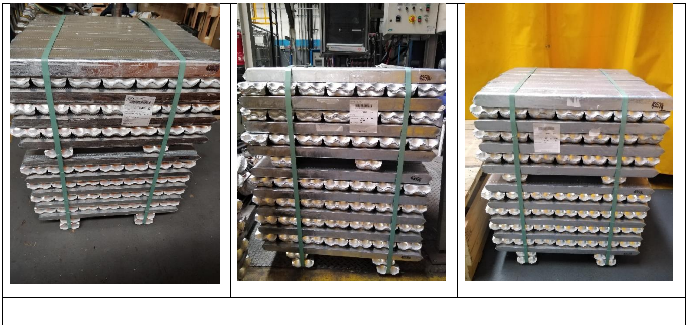
Figure 1: Pictures of the AlSi10MnMg0,3 pallets produced for the different alloy variants- from left to right Variant1 – Variant2 – Variant3
