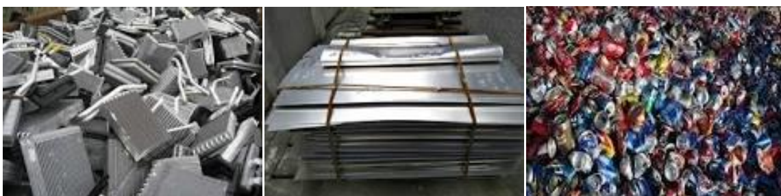
Figure 2 - From left to right: aluminium clean mixed old alloy, aluminium blind, aluminium copper radiator
