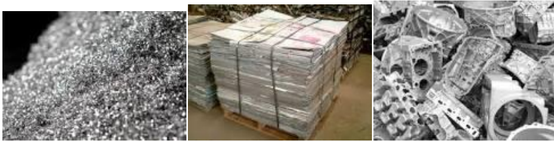
Figure 4 - From left to right: aluminium turnings, aluminium lithographic sheet, mixed aluminium castings
