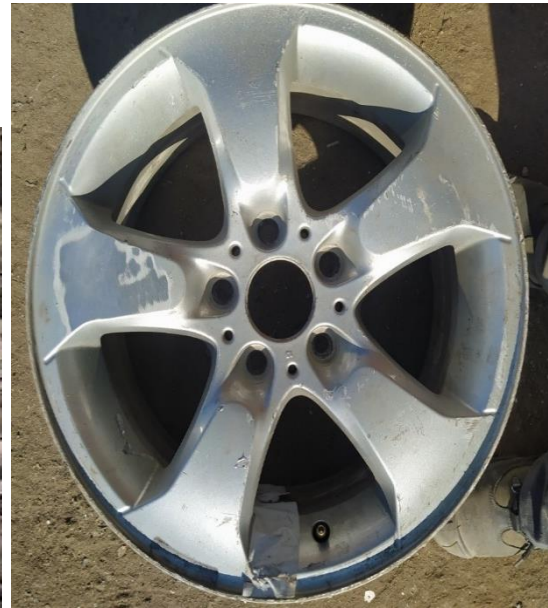
Figure 9 - End-of-life aluminium wheels dismantled from scrapped cars
