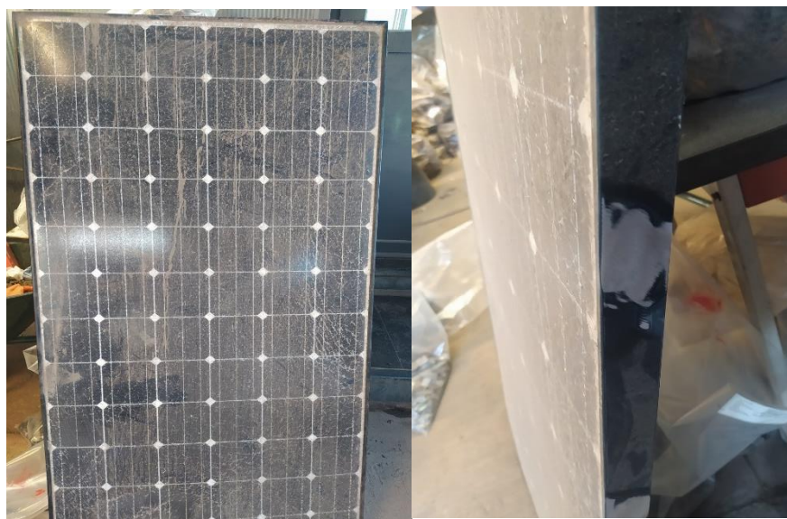
Figure 10 - End-of-life aluminium frames from scrapped photovoltaic panels
