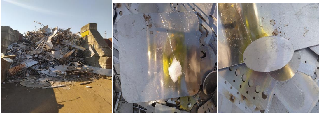
Figure 12 - Aluminium alloy-based production scraps
