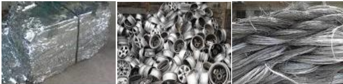
Figure 5 - From left to right: aluminium foil, aluminium rims, mixed aluminium wire and cable
