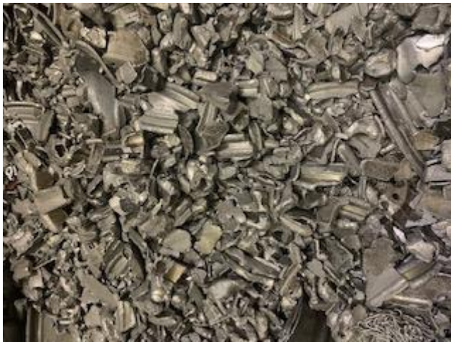
Figure 9 - End-of-life aluminium wheels dismantled from scrapped cars
