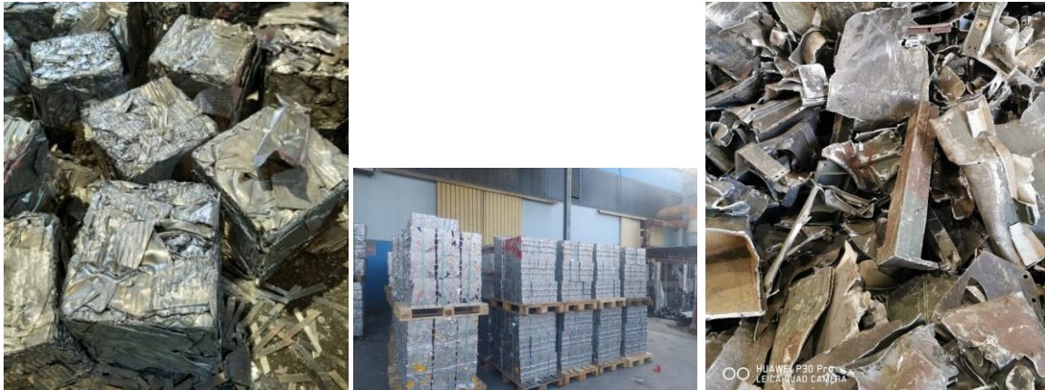
Figure 8 - From left to right: bale loose, bales on pallet, thickened pieces
