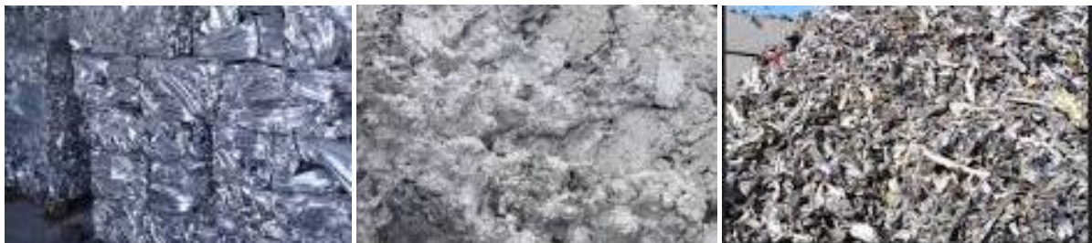
Figure 6 - From left to right: aluminium extrusion 6000 series, aluminium drosses and skimmings, zorba-shredded non ferrous scrap
