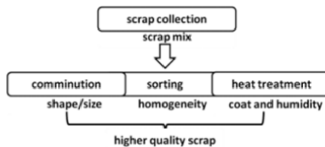
Figure 13 - From scrap mix to higher quality scrap by pre-treatment process
