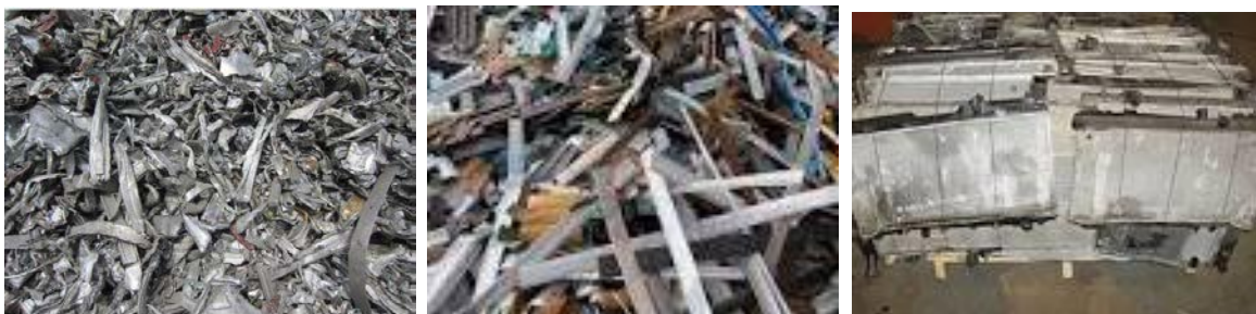
Figure 2 - From left to right: aluminium clean mixed old alloy, aluminium blind, aluminium copper radiator
