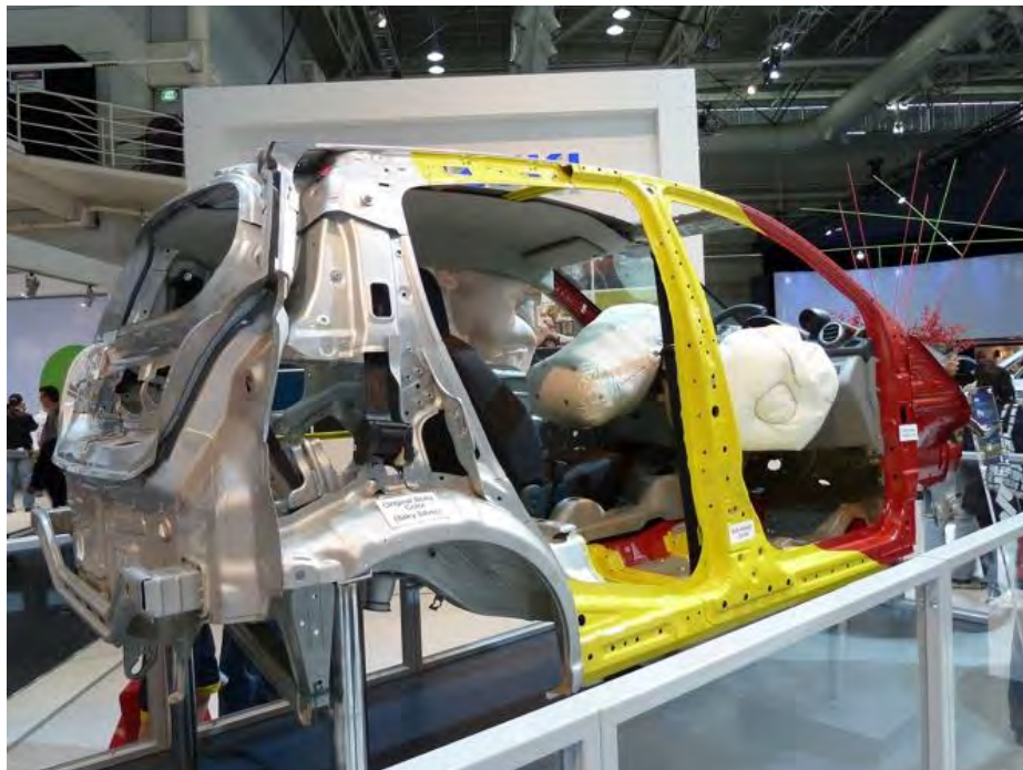
Fig. 2 – Subdivision of body-in-white into 22 components [1]
