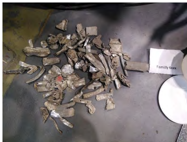
Figure 10: Image of the batch of 6xxx series scrap provided by COMET spread over the floor
