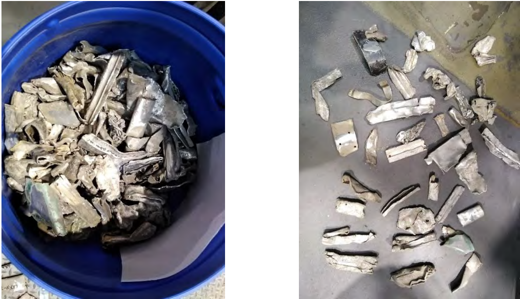
Figure 9: Image of the open barrel with the whole 5xxx series batch of scrap supplied by COMET (left) and picture of the fragments belonging approximately to 1/3 of the top of the batch spread over the floor (right)
