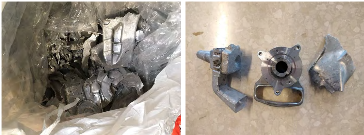
Figure 11: General image of the foundry scrap provided by Raffmetal (left) and image of 3 parts selected to conduct a chemical analysis by spectrometry (right)
