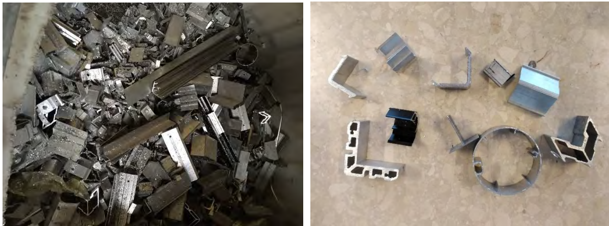
Figure 12: General overview of the 6063 extruded profile acquired from a local aluminium recycling company (left) and image of the 10 parts selected for a Spark Plasma chemical analysis (right)
