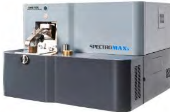
Figure 7: Image of the SPECTROMAXx F used at Eurecat to analyse the chemical composition of the selected pieces
