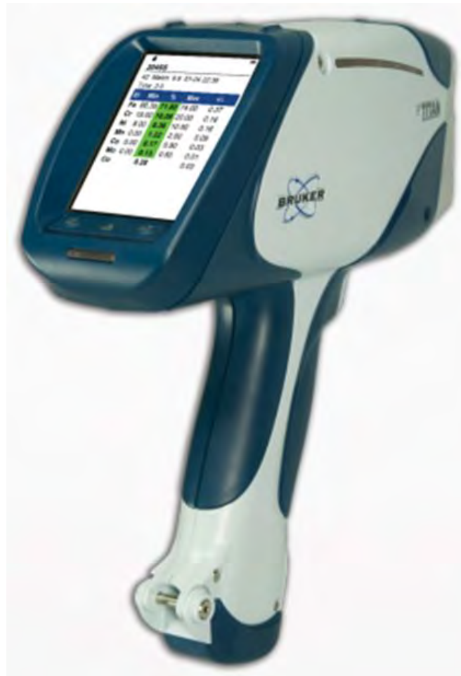
Figure 3: XRF spectrometer used for the individual analysis of (assumed) aluminium parts
