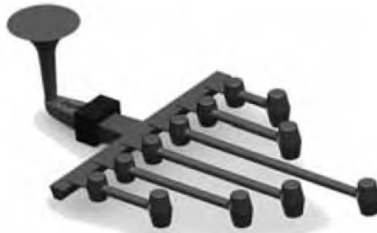
Fig. 13 – 3D-picture of dog bone shaped sand casting for HCl evaluation [23]
