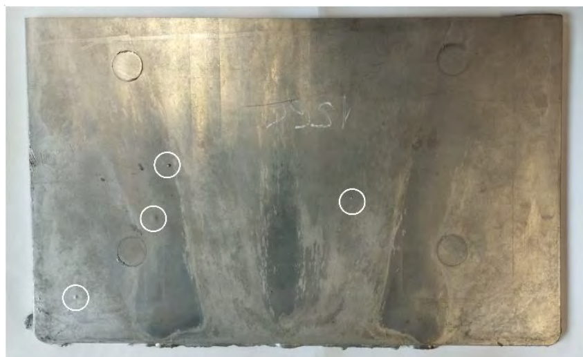
Figure 7 - Surface blisters after solution treatment
