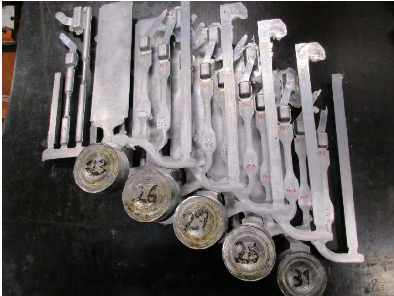
Figure 17 – Parts cast with NADIA die Hardness trends as function of time and temperature for investigated T6 conditions
