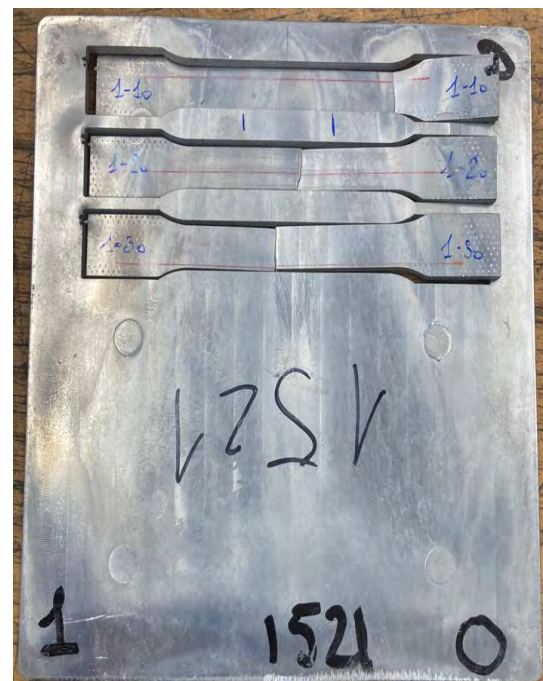
Figure 13 – Examples of specimens taken horizontally from the castings
